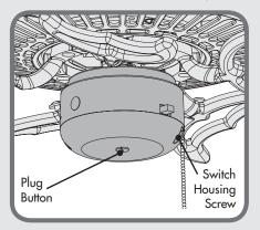
If your fan's switch housing cap resembles this one, remove the whole switch housing by removing the switch housing screws with a Phillips head screwdriver. Remove the plug button using a standard screwdriver. Then follow the TYPE-C ASSEMBLY INSTRUCTIONS on pages 8-9.
